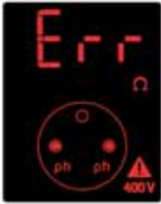
Connection between phases under 400 V.
