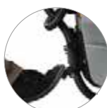
Foot pedal squeegee lifting system
