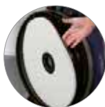
Floating integrated pad holder
