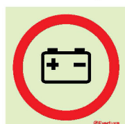
S 13 07 Emergency source of electrical power (battery)
